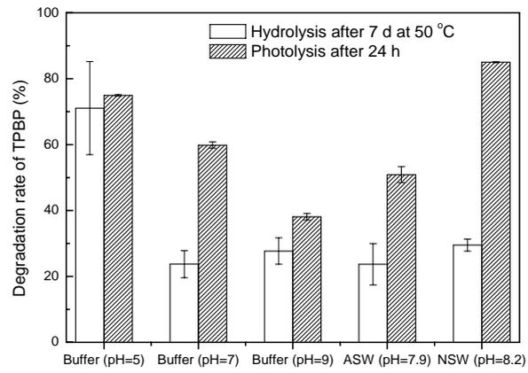
Fig. 4. Degradation rate of TPBP in the five aqueous solutions after hydrolysis and photolysis.
