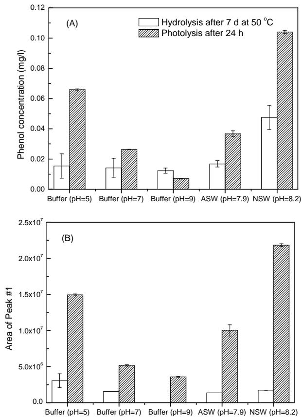
Fig. 5. Production of: (A) phenol and (B) unknown Peak #1 in the five aqueous solutions after hydrolysis and photolysis.
