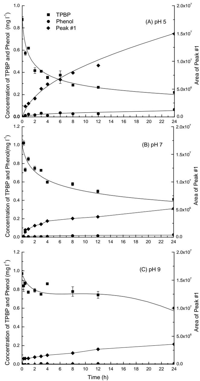
Fig. 2. Photodegradation of TPBP and the formation of phenol and the unknown Peak #1 in a sodium acetate buffer solution at: (A) pH = 5, (B) pH = 7, and (C) pH =
