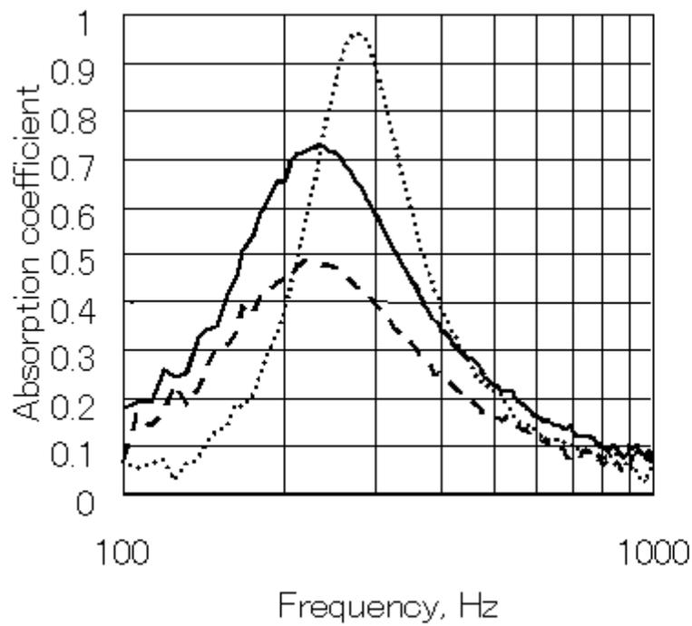
Figure 3. Results of the measured normal absorption coefficients of thick MPP specimens. All specimens are 10mm thick, and hole diameters are: 0.5mm (Specimen A: dashed line), 0.8mm (Specimen B: dotted line) and tapered hole with diameter 0.8-0.5mm (Specimen C and D: solid line. Note that the results for Specimens C and D are overlapped.).
