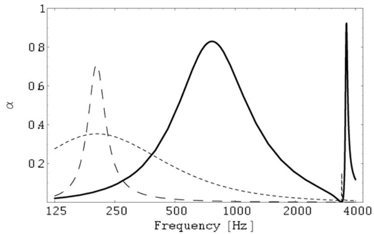
Figure 1. Numerical example of the absorption characteristics of a thick MPP calculated by Maa's theory. Hole diameter 0.4mm, thickness 0.4mm (solid line); hole diameter 0.4mm, thickness 10mm (dotted line); hole diameter 4mm, thickness 10 mm (dashed line). Other parameters: perforation ratio 1.0%, cavity depth 0.05m.
