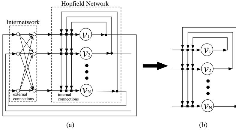
Figure 1. (a) A schematic diagram of the connections in a single-module Cross-Coupled Hopfield Nets (CCHN) with two-layer internetwork. (b) This single-module CCHN is degenerated into a simple Hopfield network as a result of the model-derivation. The white circles mean network units and the black diamonds symbolize connections of the Hopfield network.
